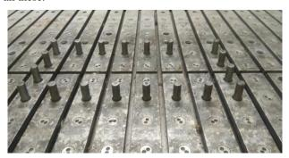
Fig.4: Cushion Pins in Bolster
