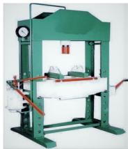
Fig.1: Manual Press Machine
